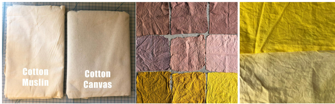
Figure 7: Left: Fabrics for testing fading. Center: original swatches with madder root and turmeric on three types of fabrics. Right top: original turmeric swatch. Right bottom: faded turmeric swatch after six and a half weeks in a window exposed to UV rays.
