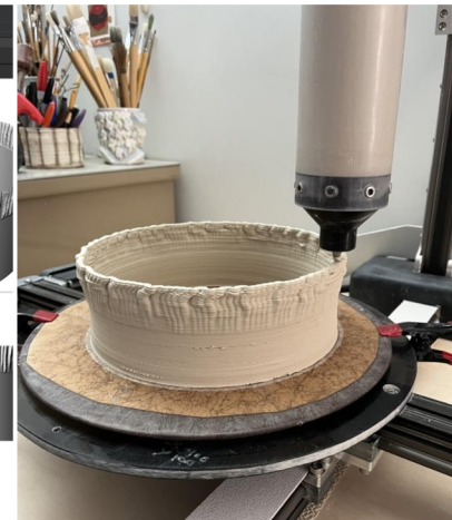
7. 3D models are 3D printed in porcelain on a PotterBot clay printer.
