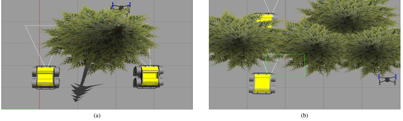
Fig. 5: Simulation environment design in Gazebo for (a) LOS, and (b) NLOS communication. The whole environment is 100\text{m} \times 100\text{m} , and each grid stands for 20\text{m} \times 20\text{m} .
