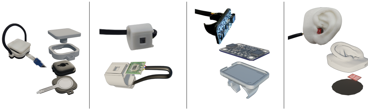
Fig. 4. (a) Weight, (b) Magnetic Field, (c) Distance, and (d) Frequency sensor units.
