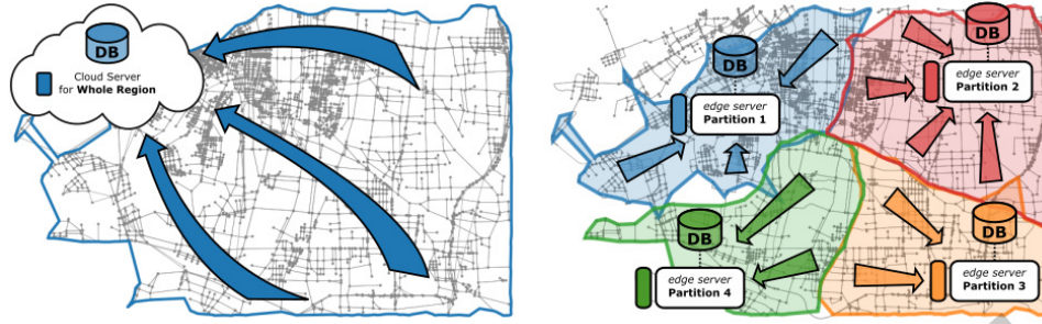
Fig. 4. Cloud-based Architecture (Left) vs Distributed/Edge-based Architecture (Right)
