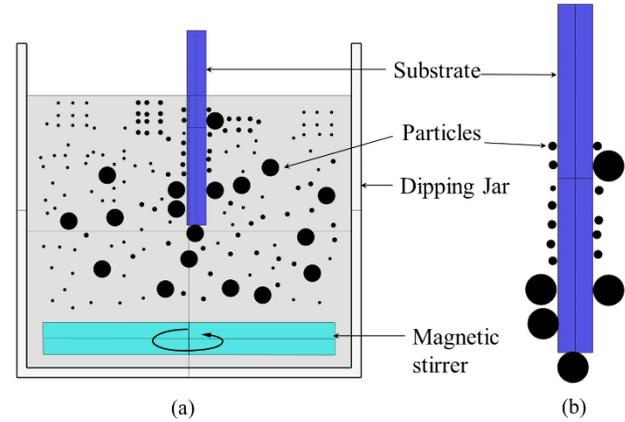
**FIGURE 1: SCHEMATIC OF THE EXPERIMENTAL SETUP (a) ROD AFTER WITHDRAWAL FROM SUSPENSION (b)**
