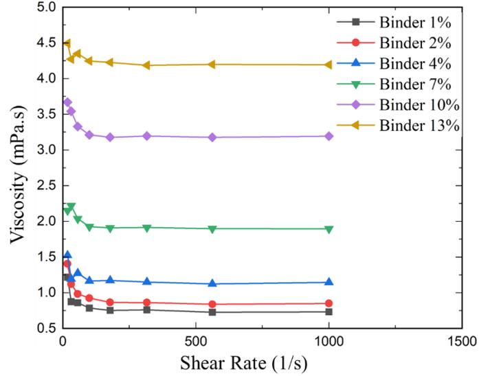
**FIGURE 2:** VARIATION OF THE VISCOSITY WITH SHEAR RATE
