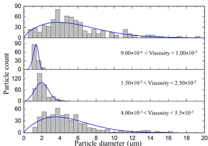
**FIGURE 5:** DISTRIBUTION OF PARTICLES AT DIFFERENT VISCOSITY RANGES
