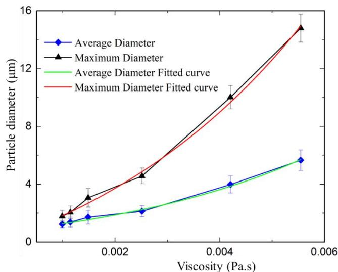
**FIGURE 4:** VARIATION OF PARTICLE SIZE WITH THE VARIATION OF VISCOSITY
