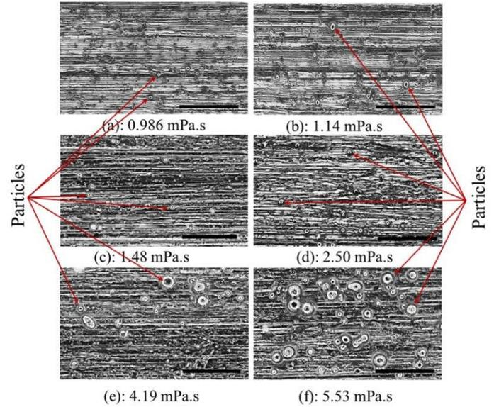
**FIGURE 3:** EXPERIMENTAL IMAGES OF THE FILTERED PARTICLES AT DIFFERENT VISCOSITIES
