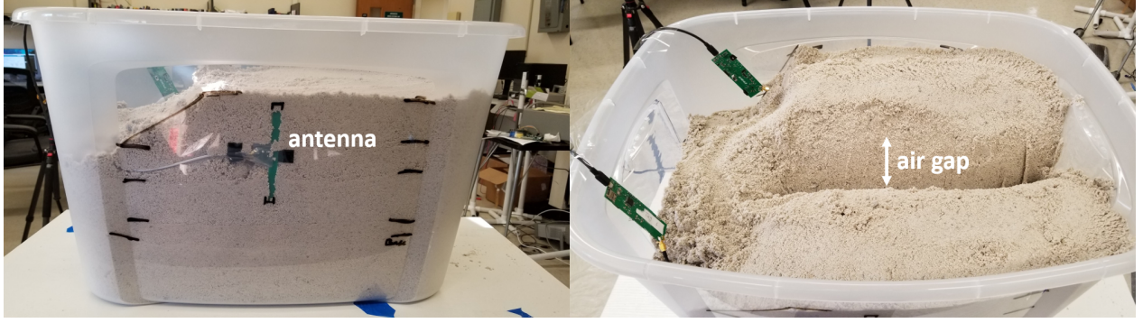
Fig. 9 – Experimental setup. Left: Side view of the antenna which is fixed to the side of the container. Right: Top view showing the air gap in the channel.
