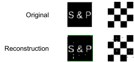
Figure 12: Pixel stealing PoC result: Original vs Reconstruction on our i7-8700 processor.
