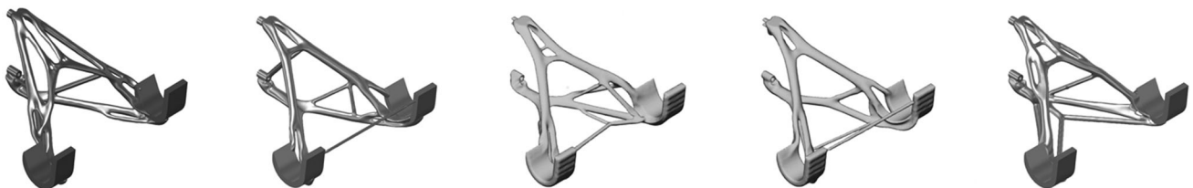
Figure 8. Computer-generated GD solutions created using Fusion 360.
