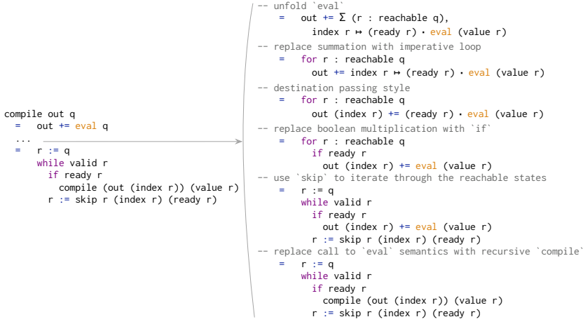
Fig. 16. A simplified version of the code generation function Figure 15 is shown on the left, along with an equational derivation for it on the right.
