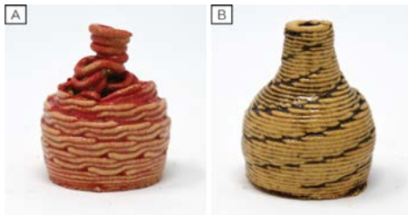
Figure 10: Surface textures generated by starting and stopping the LUTUM motor at specific points along the toolpaths. This functionality enables us to create varying patterns such as A) a wave motif and B) a staircase motif.
