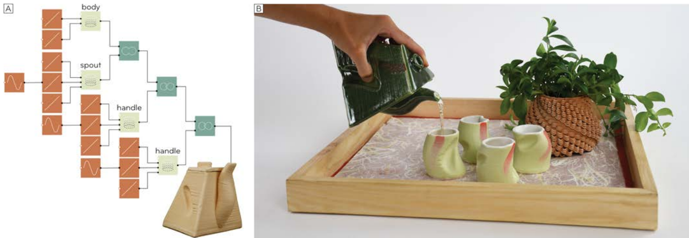
Figure 1: CoilCAM enables the design of 3D printed clay artifacts through concise, mathematically defined toolpath operations. Here we show a functional tea set created with the system. A) Schematic of the toolpath operations required to create the teapot with CoilCAM. We use a Boolean union operator to combine the body and the spout and two Boolean difference operators to generate the handle. B) Tea set with 3D printed planter demonstrating CoilCAM's ability to create surface texture.
