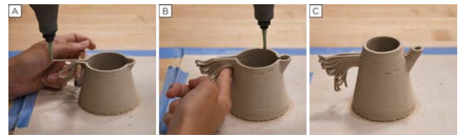
Figure 17: Human-machine collaboration. The teapot is designed with a gravity-shaped handle. The craftsperson uses A) a tool and B) a finger to support the handle and create an opening as shown in C.
