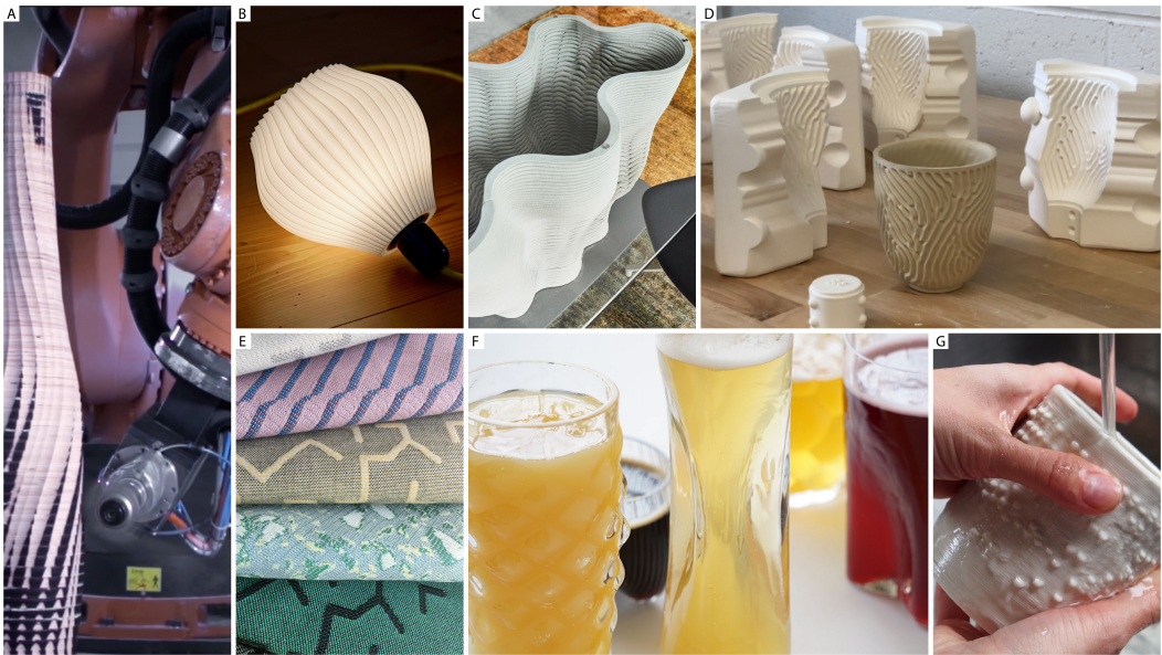
Fig. 1. Products made with workflows that included digital fabrication steps. We examined products made with different materials including wood, concrete, glass, fabric, plastic, and porcelain. A: Robotically milled wooden vase by ODK Design, B: 3D printed pendant lamp by CW&T, C: 3D printed concrete table by Fritsch+Durisotti, D: slip cast porcelain cup with plaster mold by Nervous System, E: Jacquard woven textiles by WOVNS F: craft beer glasses by Path Design, and G: 3D printed clay cup by Slip Rabbit.
