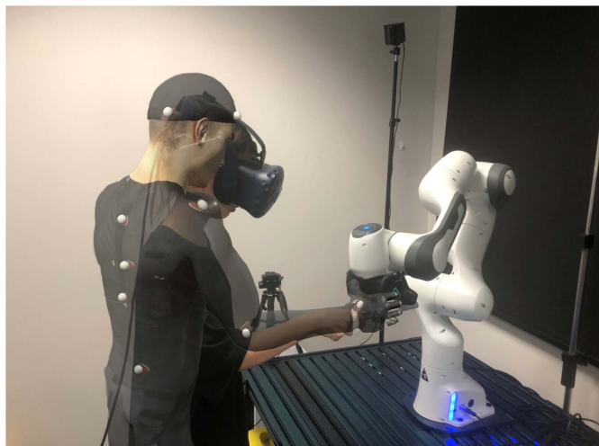
Fig. 5. Robotic system simulates a virtual tutor grabbing a trainee's hand/limb, creating an embodied training experience.
