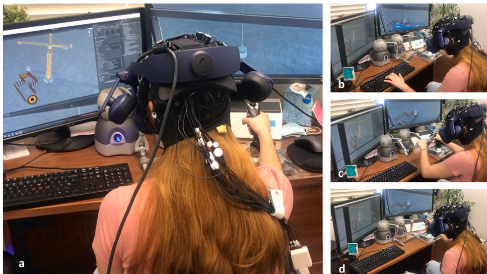
Fig. 11. A participant in the tower crane material handling experiment under four conditions. a. Control. b. Reverse. c. Haptic. d. Automatic
