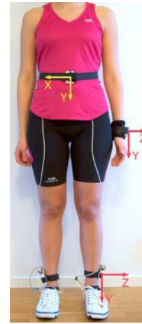
FIGURE 1. Position and orientation of four accelerometer sensors used in MAREA database [9]. (Figure courtesy of Dr. Siddhartha Khandelwal and Prof. Nicholas Wickström.)
