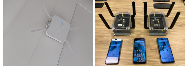
(a) RU installed on ceiling
