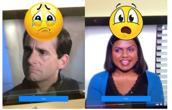
Fig. 16. The trained EfficientNetV2 MLModel emoticon results in the iPad showing a (left) correct “sad” emotion classification, and (right) an incorrect “surprise” emotion classification.
