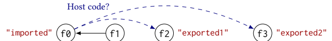
(b) Simplified call graph for (a). The presence of the blue dashed edges depends on (assumptions about) the host code of f0.
