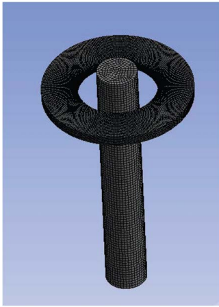
Fig. 2 ANSYS AQWA model for calculation of hydrodynamic coefficients
