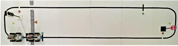
Fig. 2: Physical platform showing the leading, following vehicle, Road Side Unit (RSU), and traffic signs.
