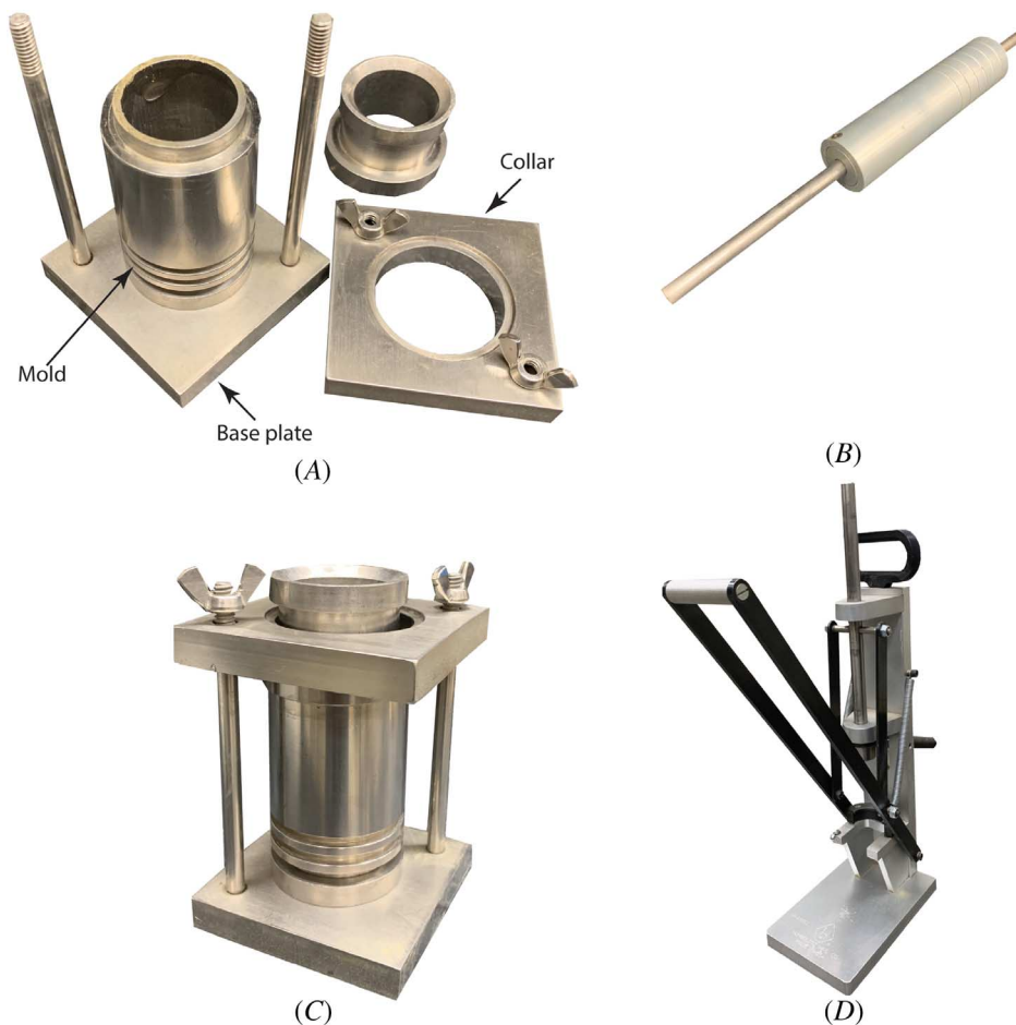
FIG. 4 (A) Harvard miniature compaction equipment, (B) tamper assembly, (C) mold assembly, and (D) specimen ejector.
