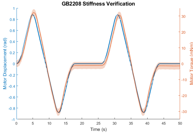
Fig. 5. An example of the prescribed KUKA end-effector rotation to induce the motor displacement and the measured torque produced by the GB2208 motor. The torque presented here is the difference between the average measured torque with a stiffness of 30 mNm/rad and the average measured torque for the three control trials. The orange highlighted region shows the standard deviation of the measured torque.
