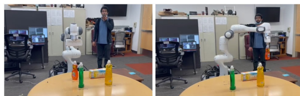
Figure 1: Left: User giving speech commands through the mobile application. Right: Robot performing the task based on the speech command
