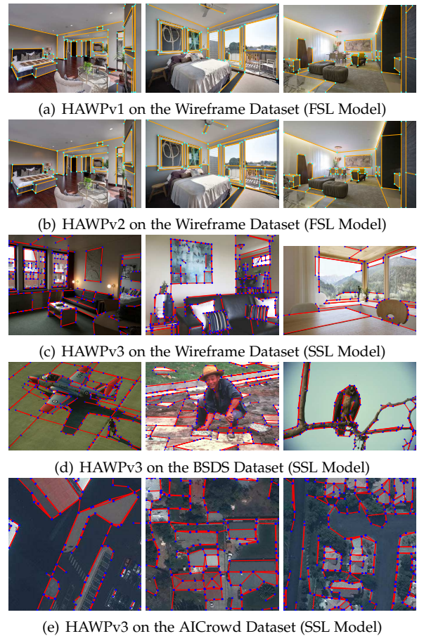
Fig. 1. The proposed HAWP models excel in wireframe structure perception using both fully-supervised learning (FSL) and self-supervised learning (SSL). HAWPv1 [23] and improved HAWPv2 are FSL models trained with human-annotated wireframes, primarily in indoor images. HAWPv3, an SSL model built on HAWPv2, enables wireframe parsing in out-of-distribution images such as those from the BSDS-500 dataset [8] and AICrowd dataset [24], without requiring labeled wireframes.
