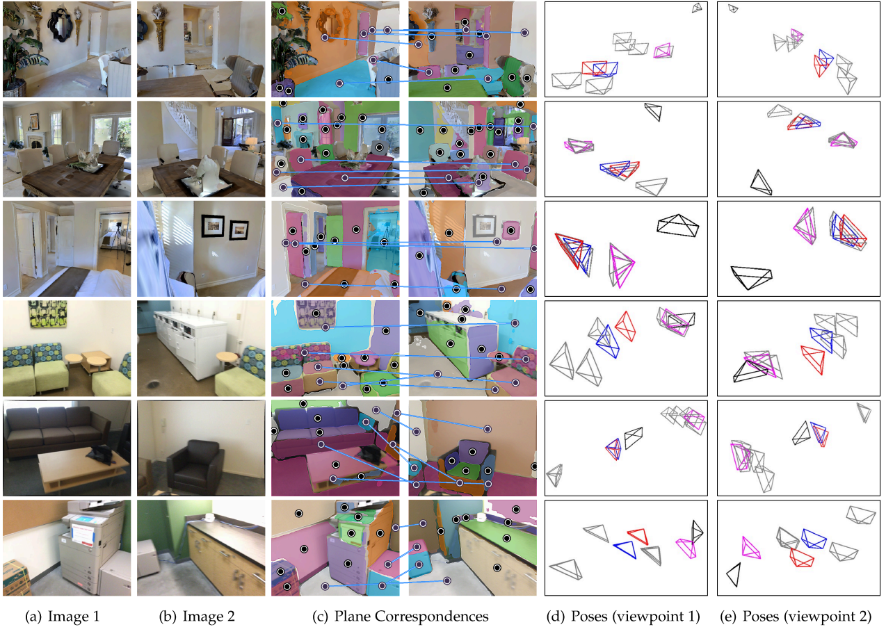
Fig. 6. Qualitative results of the refined poses and plane correspondences on the Matterport3D [13] dataset (first three rows) and the ScanNet [14] dataset (last three rows). The Pink , Blue and Red frustums show the initial, the refined, and the ground truth cameras of the first image respectively. Gray frustums show the one-plane pose hypotheses of the first image generated from plane correspondences. Black frustums show the camera of the second image.
