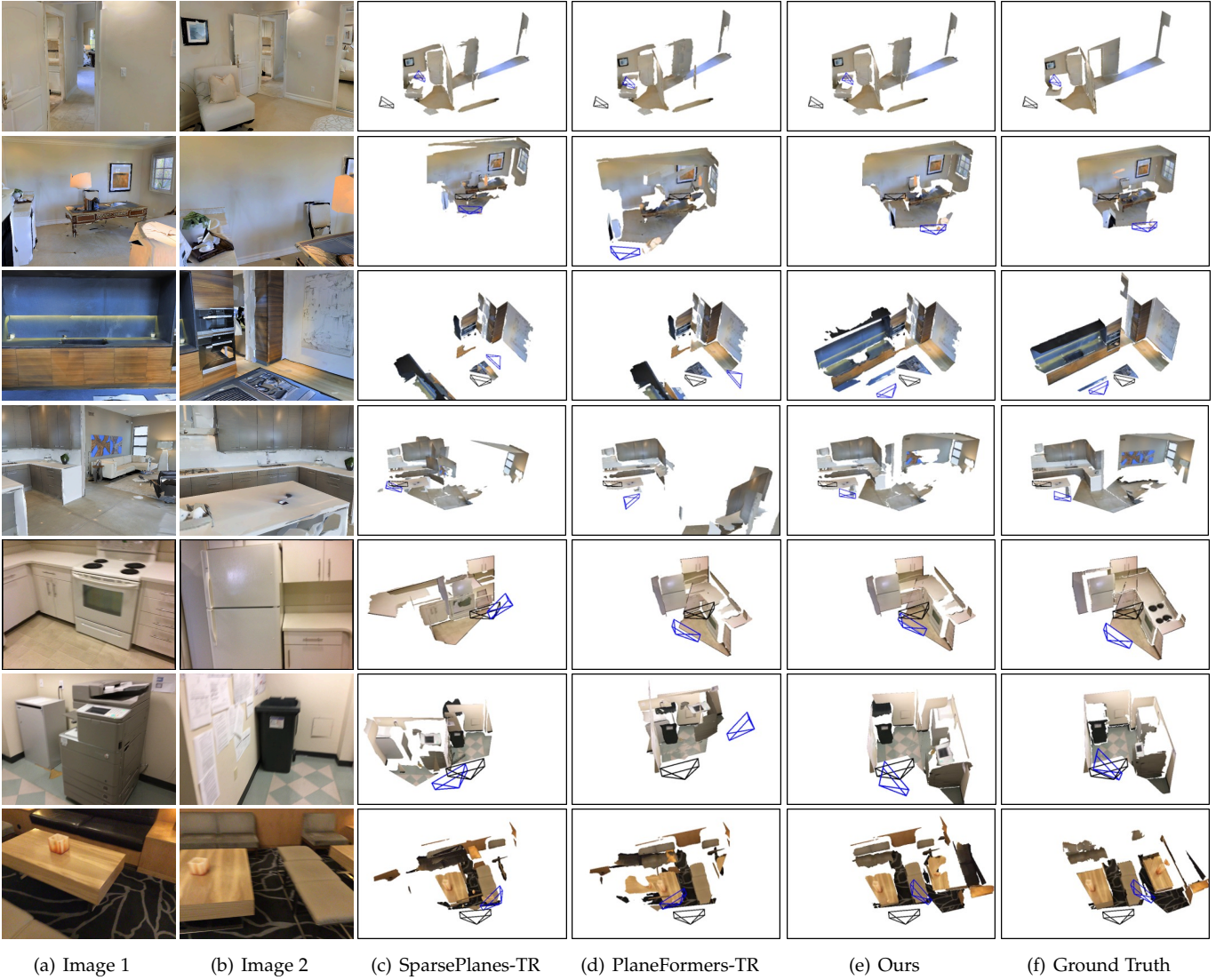
Fig. 7. Comparison of 3D plane reconstruction results on the Matterport3D [13] dataset (first four rows) and the ScanNet [14] dataset (last three rows). Blue and Black frustums show cameras of the first and the second images respectively.
