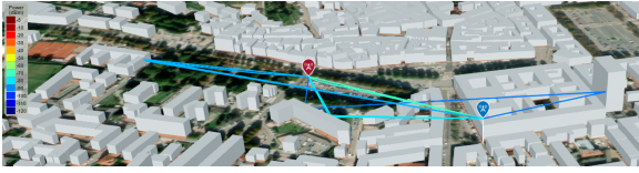
Fig. 4: Ray tracing with multiple propagation paths between the transmitter and the receiver.
