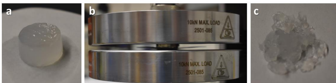
Figure 3. Steps of the compression tests: a) Hydrogel placed on filter paper before compression; b) Ongoing compression testing of hydrogel; c) Appearance of hydrogel after compression
