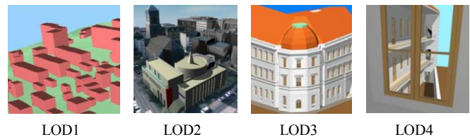
Figure 1. Four levels of detail building structures [2].
