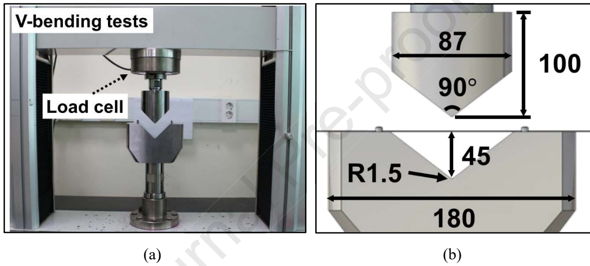
Figure 4: Experimental setup used for the V-bending tests: (a) test machine and incorporated tools and (b) specific dimensions of the tools [69,70]
