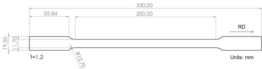
Fig. 2. Specimen geometry for CBT experiments.
