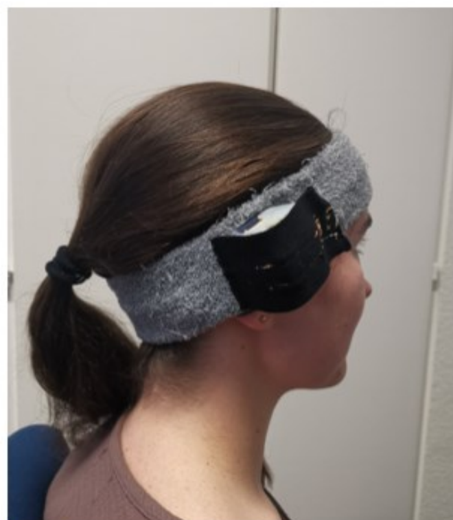
Figure 2 The Auracle: eating recognition system.
