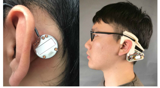
Fig. 11. Left panel: a contact microphone was used to collect acoustic data from the mastoid bone as study participants performed various eating and non-eating tasks [6]. Right panel: prototype of the complete wearable device that we are developing for dietary monitoring [7].
