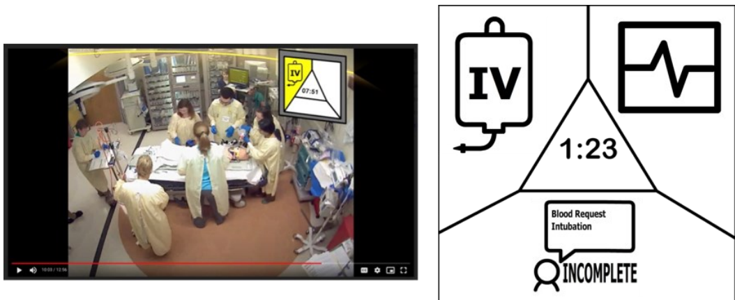
Figure 3: Components of the finalized prototype alert system. Left: A collage showing the system overlaid on top of a simulation video to illustrate the system (grid with alerts and ceiling lights) in the room. Right: A zoomed-in grid component showing the alerts for No IV access (upper left), No vital signs (upper right), Incomplete request (bottom), and Time interval (center).
