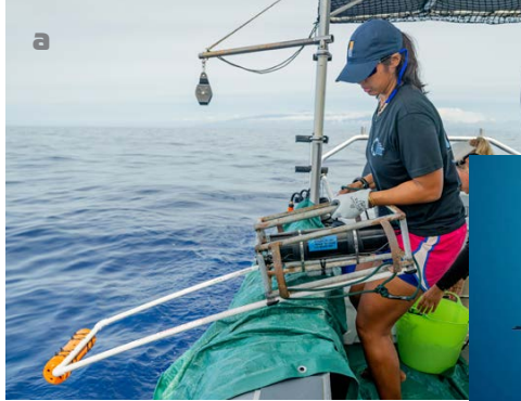
FIGURE 3. (a) A baited remote underwater video (BRUV) is deployed from a small boat. (b) This Galápagos shark was recorded using a BRUV.
