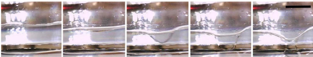
Fig. 4: Evolution of droplet formation in the TaFISA channel. The scalebar shown is 1 cm
