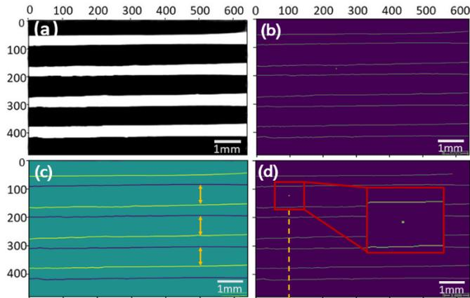
**FIGURE 5:** WIDTH MEASUREMENT PROCESS: (A) GREYSCALE IMAGE; (B) APPLY CANNY ALGORITHM TO GREYSCALE IMAGE; (C) APPLY SOBEL FILTER TO GREYSCALE IMAGE; (D) CANNY MAP WITH NOISE ON FIRST DETECTING COLUMN.
