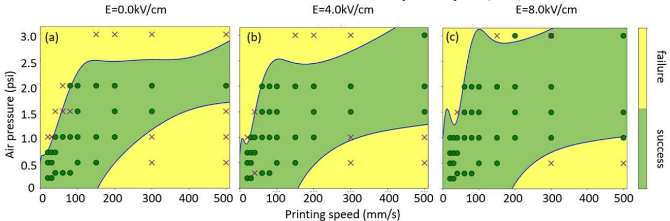
**FIGURE 6:** PRINTING RESULT PREDICTION FROM MLP CLASSIFIER MODEL
