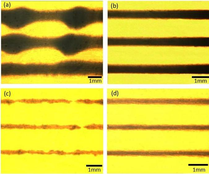
**FIGURE 3:** (A) BULGE SAMPLE; (B) BULGE ISSUE SOLVED BY ADDING 8KV/CM ELETRIC FIELD; (C) DISCONTINUOUS SAMPLE; (D) DISCONTINUOUS ISSUE SOLVED BY ADDING 8KV/CM ELETRIC FIELD.
