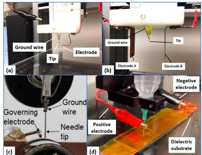
**FIGURE 1:** EDIW SETUP DESIGN: (A) GOVERNING ELECTRODE IN FRONT AND GROUND WIRE ON TIP [7]; (B) ELECTRIC FIELD AROUND TIP [4]; (C) GOVERNING ELECTRODE ON TOP OF BALL-BEARING [9]; (D) ELECTRODES ON TIP AND SUBSTRATE
