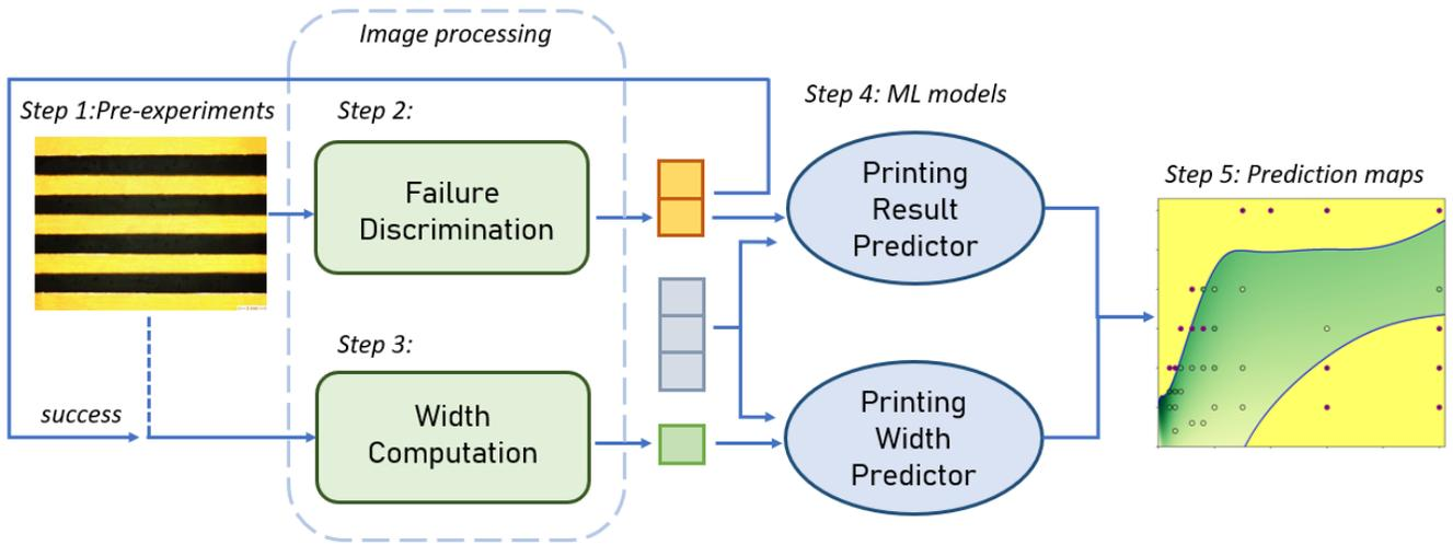
**FIGURE 2:** FLOW CHART OF A DATA DRIVEN PREDICTIVE MODELING SYSTEM TO PREDICT THE PRINT QUALITY AND PRINTING WIDTH
