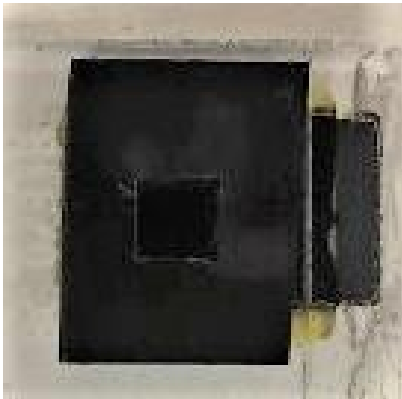
Fig. 9. Cell with carbon mask to reduce active area from 0.49 cm² to 0.09 cm².
