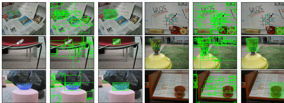
Fig. 9 Instance identification on the SIVAL-25-deep dataset across different classes. In each set of three pictures the leftmost is the original image, the middle shows the bag of patches extracted by the EdgeBox detector, and the final image highlights the patch identified by our approach for classifying the image
