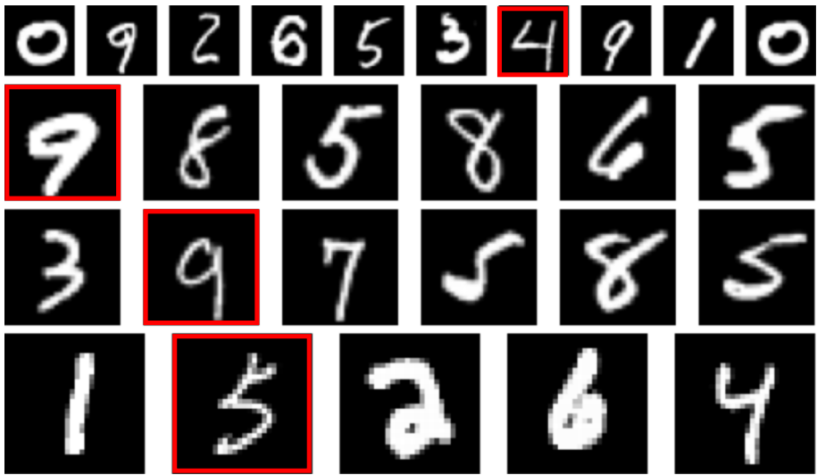
Fig. 7 Instance identification results on the first five testing bags of our method on the MNIST-bags dataset with the detectors in Fig. 6. Our approach correctly classifies the first, second and third bags. Although the first bag is classified correctly the “9”s are not properly identified
