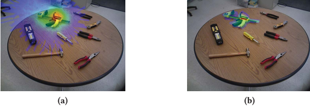
Figure 7: Static frame 6 DoF pose estimation with PMPNBP, (a) represents the initial random sampled belief of the clamp object and (b) shows the convergence of samples after 100 iterations of belief message passing.
