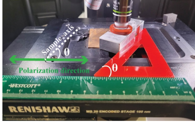
Figure 3. An example of PRS measurement at a polarized angle \theta of 60^\circ . The glass slide was glued on an aluminium holder and the rubber gasket was used to immerse the ETS samples in PBS. The polarization angle was incremented by 30^\circ while rotating the holder using the 30/60degree set square.
