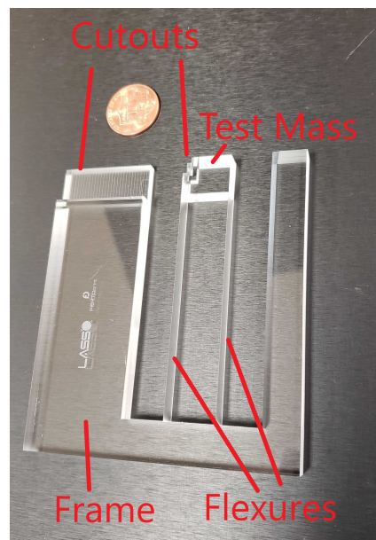
Figure 1. A diagram of our 5 Hz resonator. A penny is added for reference.
