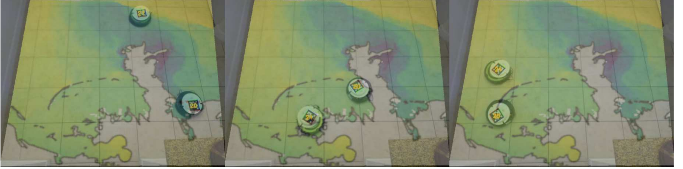
Fig. 3: Physical experiment with multiple robots: Two robots are collecting information from a projected spatial field.
