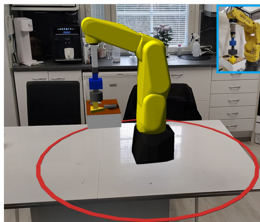
Figure 7. Augmented Reality with visualization of robot working area.
