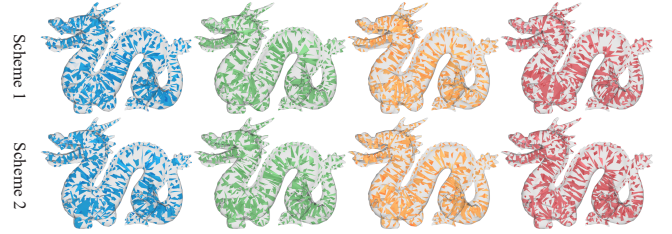
Fig. 5. Complementary coloring. Our hybrid sweep is used with a complementary coloring strategy. The coloring of stencils is pre-computed, and we generate multiple color schemes to make sure each stencil shows up in an independent color group at least in one scheme. Here, we show first four colors of two schemes on a dragon model.
