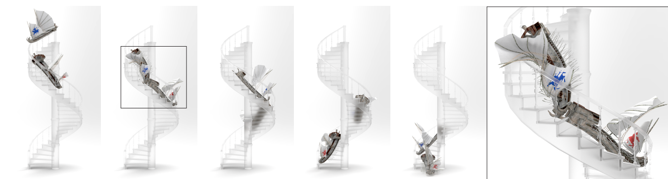
Fig. 1. Falling barbarian ships. We propose a new GPU-based algorithm for generic finite element simulation using interior-point methods. Due to the use of barrier functions, interior-point methods are expensive, and the requirement of per-iteration CCD imposes extra challenges for GPU parallelization. Our method is locally second-order leveraging complex-step finite difference to efficiently estimate local Hessian-vector products. We design a complementary coloring and hybrid sweep scheme to fully exploit the throughput of the GPU. Together with a dedicated warm-start process, our method offers speedup of two orders, even with intense contacts and collisions. As a demonstration, the teaser figure shows snapshots of two barbarian ships falling on a spiral stair. There are nearly one million (974K) elements on the ships. The thin paddles at both sides collide with the staircase and the handrails yielding rich and interesting deformations. Under the time step of \Delta t = 1/100 sec, our simulation faithfully captures all the details but it is 129\times faster than the vanilla CPU IPC [Li et al. 2020]. Indeed, our GPU simulation is faster than the state-of-the-art reduced simulation [Lan et al. 2021]. The simulation remains efficient and robust even after we increase the time step size to \Delta t = 1/30 sec.
