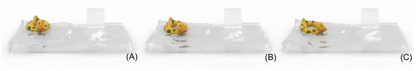
Fig. 5. Bob simulated with (A) Joint Optimization, (B) Time Splitting with Contact Proxy, and (C) Baseline Time Splitting. For this example, baseline time splitting can also produce visually plausible results, and our proxy-assisted scheme is 3× faster than joint optimization.
