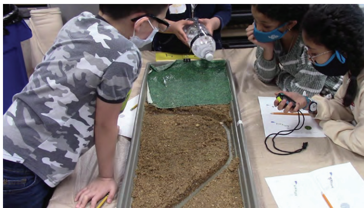
Figure 2a (left). A student group testing a (a) pervious surface on the stream table. The student at the top of the images is the "rain maker," adding water using a modified 2L rain bottle on pervious surface uphill of the river. Other student roles include: the "water watcher," who observes where the water is going and verbalizes how water is moving through the model; the "river watcher," who verbalizes when the sawdust (located midstream) moves to indicate the river has started flowing and the timer should be stopped and the "time-keeper," who times the trial from when the "rain" starts until the river starts flowing. Safety Note: Since students were working with water, each group had a towel to clean up any spills. Students were instructed not to touch the wet sand or sawdust for safety reasons. Photo Credit: L. Mossa, AGI
