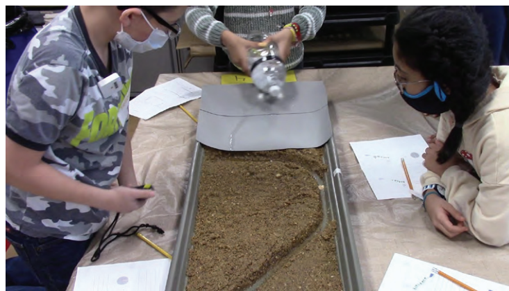
Figure 2a (left). A student group testing a (a) pervious surface on the stream table. The student at the top of the images is the "rain maker," adding water using a modified 2L rain bottle on pervious surface uphill of the river. Other student roles include: the "water watcher," who observes where the water is going and verbalizes how water is moving through the model; the "river watcher," who verbalizes when the sawdust (located midstream) moves to indicate the river has started flowing and the timer should be stopped and the "time-keeper," who times the trial from when the "rain" starts until the river starts flowing. Safety Note: Since students were working with water, each group had a towel to clean up any spills. Students were instructed not to touch the wet sand or sawdust for safety reasons. Photo Credit: L. Mossa, AGI
