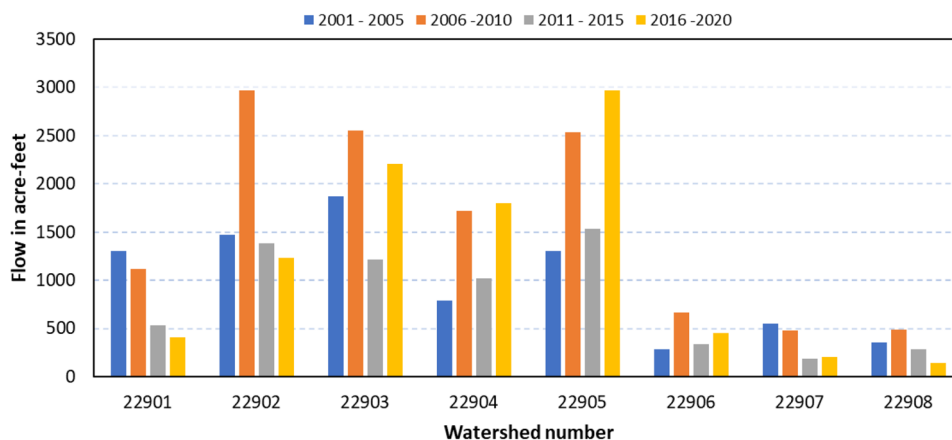
Fig. 13 Five-year increments of ungauged monthly mean flow values calculated from four different periods of record (time periods from 2001–2005, 2006–2010, 2011–2015, and 2016–2020) for the eight different LLM sub-watersheds. Watershed numbers and respective surface
