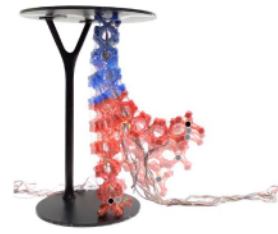
Fig. 7. Maximum reach of the arm in the x direction; black dots show a point on the center of the end effector).
