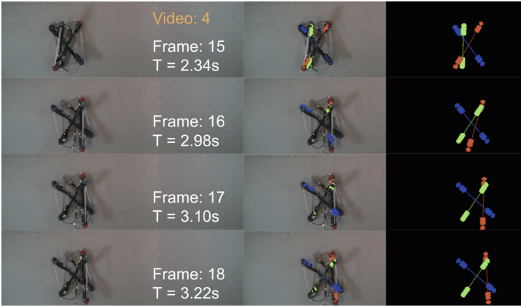
Fig. 8. Failure case. A large tracking error occurs at the frame 16 of this video. The robot has a significant movement between two consecutive frames and not enough iterations were performed to make the estimates converge. Tracking is fully recovered later at frame 18.
