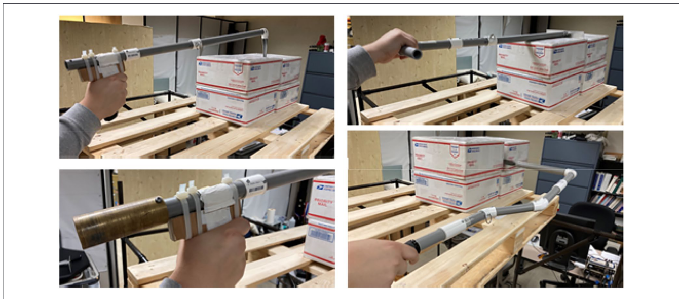
Figure 6. Examples of the box pulling task with the different handle and tip designs.
