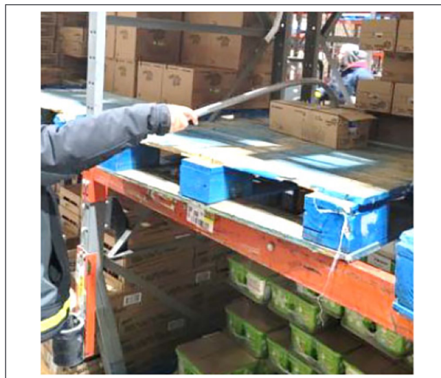
Figure 2. A case hook being used to access a 2 nd tier case.
