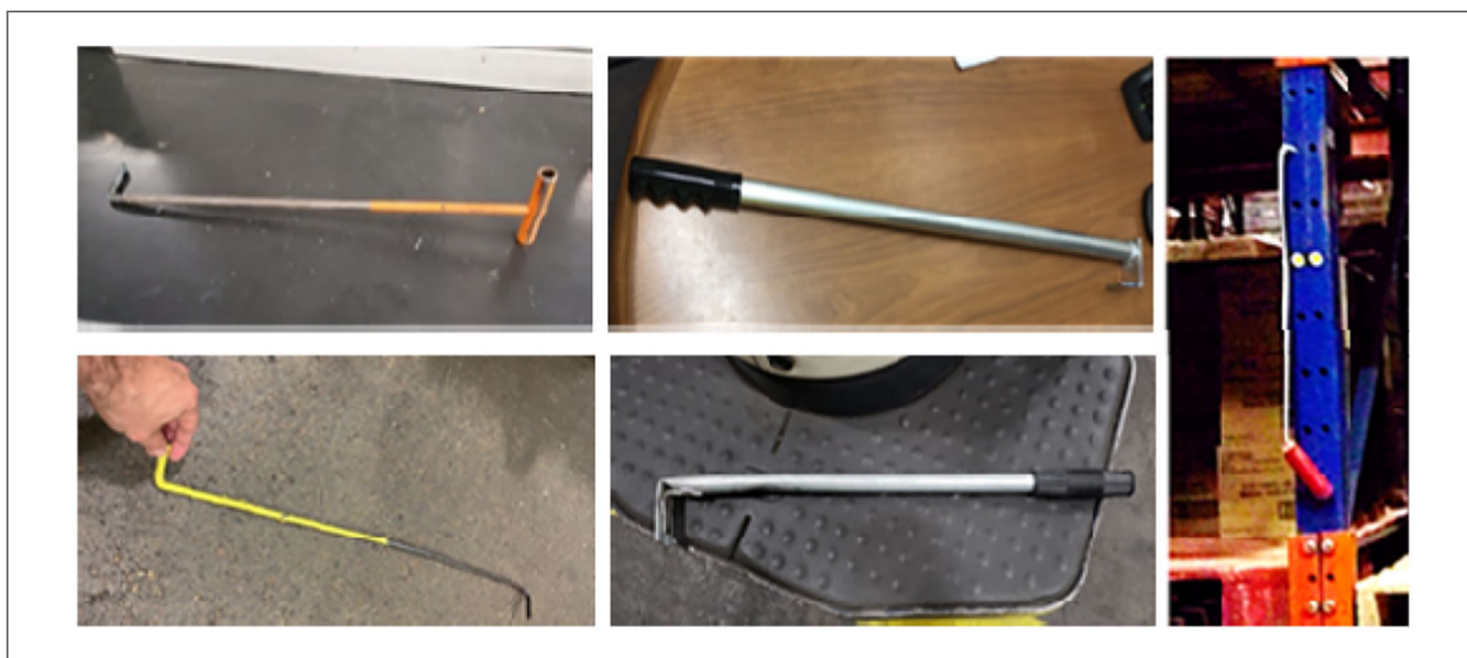
Figure 3. Examples of case hooks currently used in grocery distribution centers.
